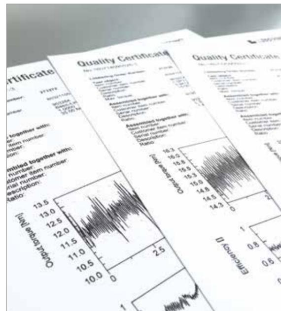
Right: The quality certificate with all relevant data for the later calibration of the fastening system.
